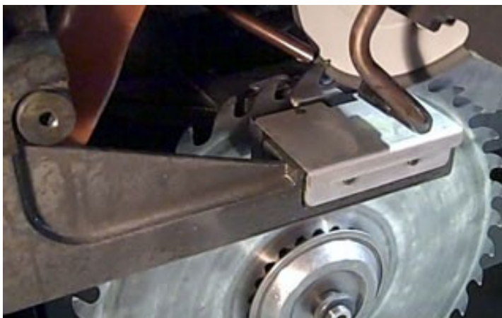
CA100 sharpens special 36 tooth circular saw
