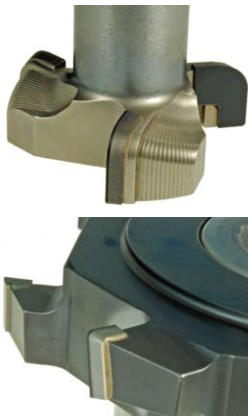
The company uses the disc-erosion machine's grinding capabilities to grind the secondary clearance behind a tool's diamond tip. Note the difference in surface finishes between the secondary on the left created via EDM and the secondary below created by grinding.
