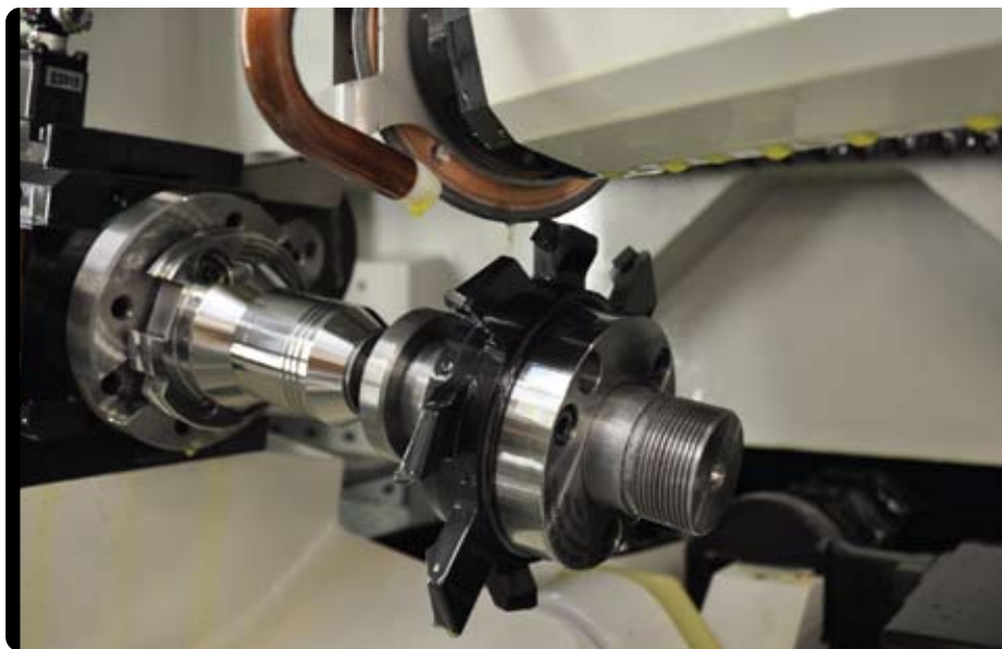
The company uses the disc-erosion machine's grinding capabilities to grind the secondary clearance behind a tool's diamond tip. Note the difference in surface finishes between the secondary on the left created via EDM and the secondary below created by grinding.
