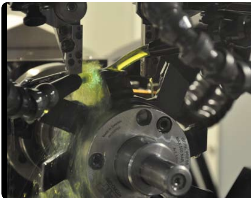
Right The tool manufacturer first adopted horizontal wire EDM so it could enter the PCD tool market. Horizontal wire orientation, adjustable guides and five-axis motion allow these machines to produce complex, multiple-wing profile tools.
