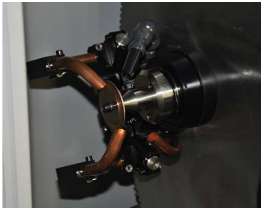
This six-station tool changer can store and automatically change wheel packs for the disc-erosion machine's electrodes and grinding wheels.
