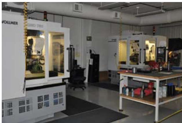
Right The tool manufacturer first adopted horizontal wire EDM so it could enter the PCD tool market. Horizontal wire orientation, adjustable guides and five-axis motion allow these machines to produce complex, multiple-wing profile tools.
