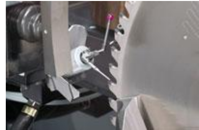
The Vollmer erosion machining center measures the dimensions for teeth of a PCD blade.
